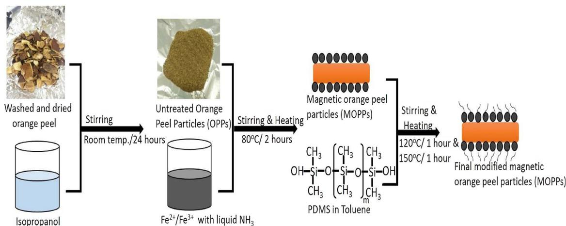
Fig. 1. Schematic diagram for the synthesis of highly hydrophobic modified magnetic orange peel particles (MOPPs) from waste materials (orange peel).
