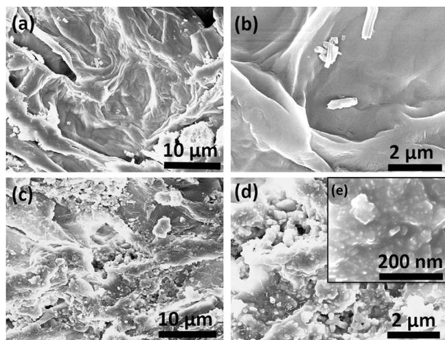
Fig. 3. SEM images of untreated orange peel particles in (a) low and (b) high magnification and SEM images of modified magnetic orange peel particles in (c) low, (d) high and (e) very high magnification.
