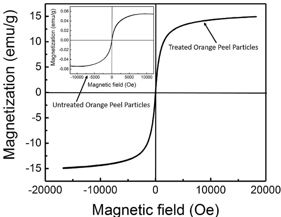
Fig. 8. VSM measurement result of pristine orange peel particles and PDMS coated magnetic orange peel particles.
