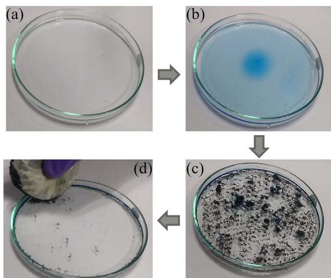
Fig. 9. Diesel oil removal from the water surface with the help of hydrophobic and superoleophilic magnetic orange peel particles under the magnetic field. The diesel oil was coloured with blue dye for clarity.
