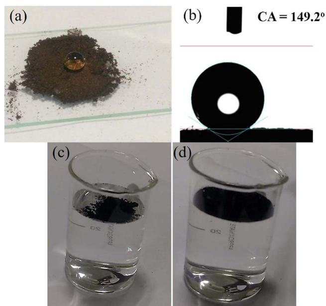
Fig. 6. (a) Digital photograph image of water droplet placed on the surface of modified MOPPs, (b) optical image of water droplet placed on that surface, (C) digital photograph image of modified MOPPs on the surface of water before and (d) after vigorous agitation.
