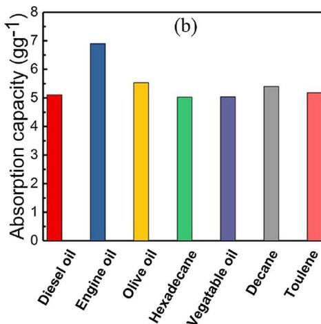
Fig. 10. (a) Oil-absorption capacity ( $Q$ ) for the PDMS modified MOPPs as a function of removal time and (b) absorption capacities of the modified MOPPs for different oils and organic solvents in terms of weight of the particles.
