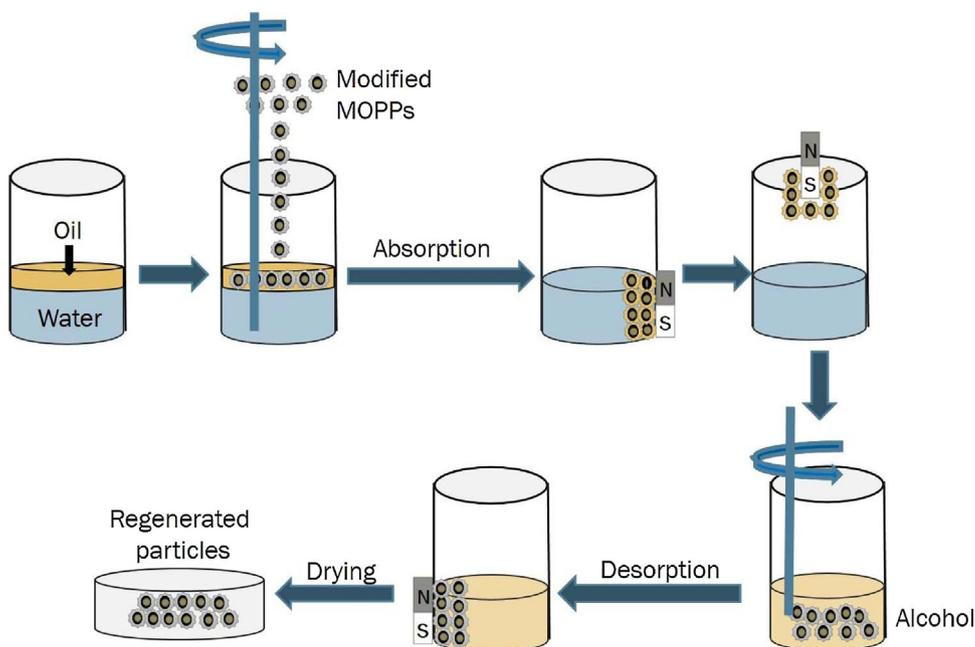
Fig. 2. Illustration for the removal oil from the surface of water by using hydrophobic and superoleophilic MOPPs under the external magnetic field and their recycle route.
