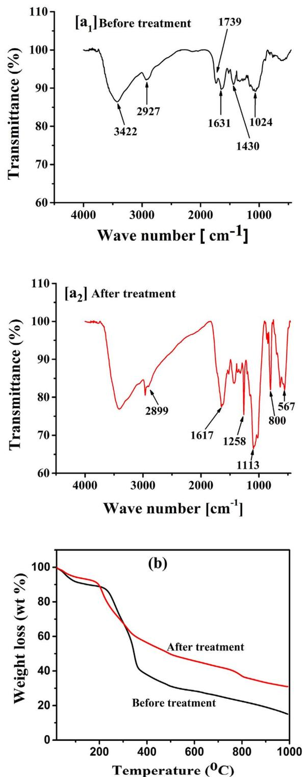
Fig. 5. (a) FTIR spectra of untreated orange peel particles (a<sub>1</sub>-before treatment) and final modified orange peel particles (a<sub>2</sub> after treatment) and (b) TGA curves of orange peel particles before treatment and after treatment.
