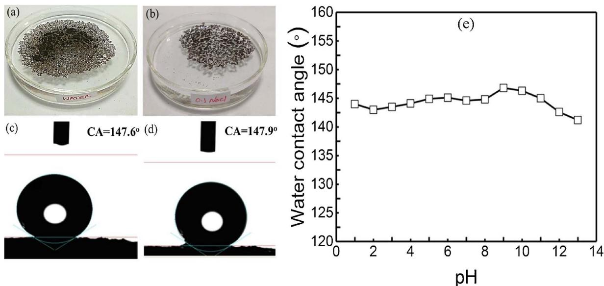
Fig. 7. Digital photograph image of modified MOPPs after floating for 24 h on (a) water surface, (b) aqueous solution of 0.1 M NaCl, and their optical image after floating for 24 h on (c) water surface and (d) aqueous solution of 0.1 M NaCl, (e) water contact angles of modified MOPPs after floating over the aqueous solution for 24 h with pH ranging from 1 to 13.
