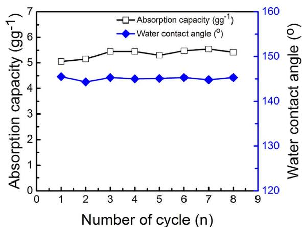
Fig. 11. Water contact angle and oil-absorption capacity of the modified MOPPs after different water-oil separation cycles.
